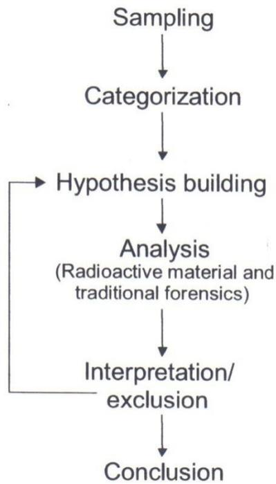
**Figure 2 – Nuclear forensics fingerprinting process <sup>(7)</sup>.**
