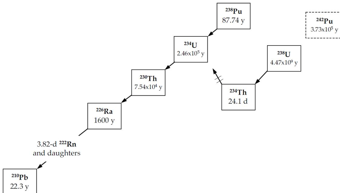
**Figure 3- Radio-chronometer used in nuclear forensics investigations <sup>(4)</sup>.**
