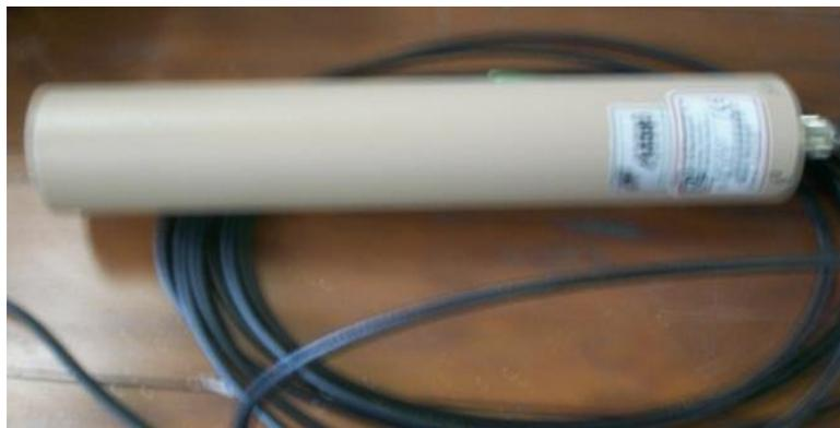
**Figure 3: NaI scintillator of 2", Ludlum, model 44-10.**
