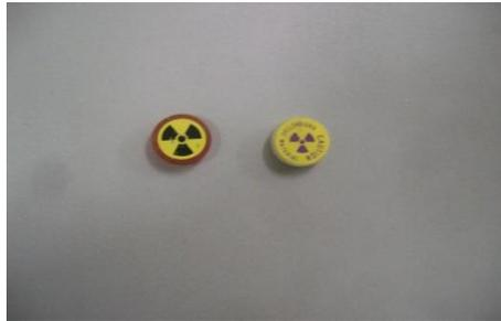
**Figure 2: Models of radioactive sources used (Am-241-left; Cs-137-right).**
