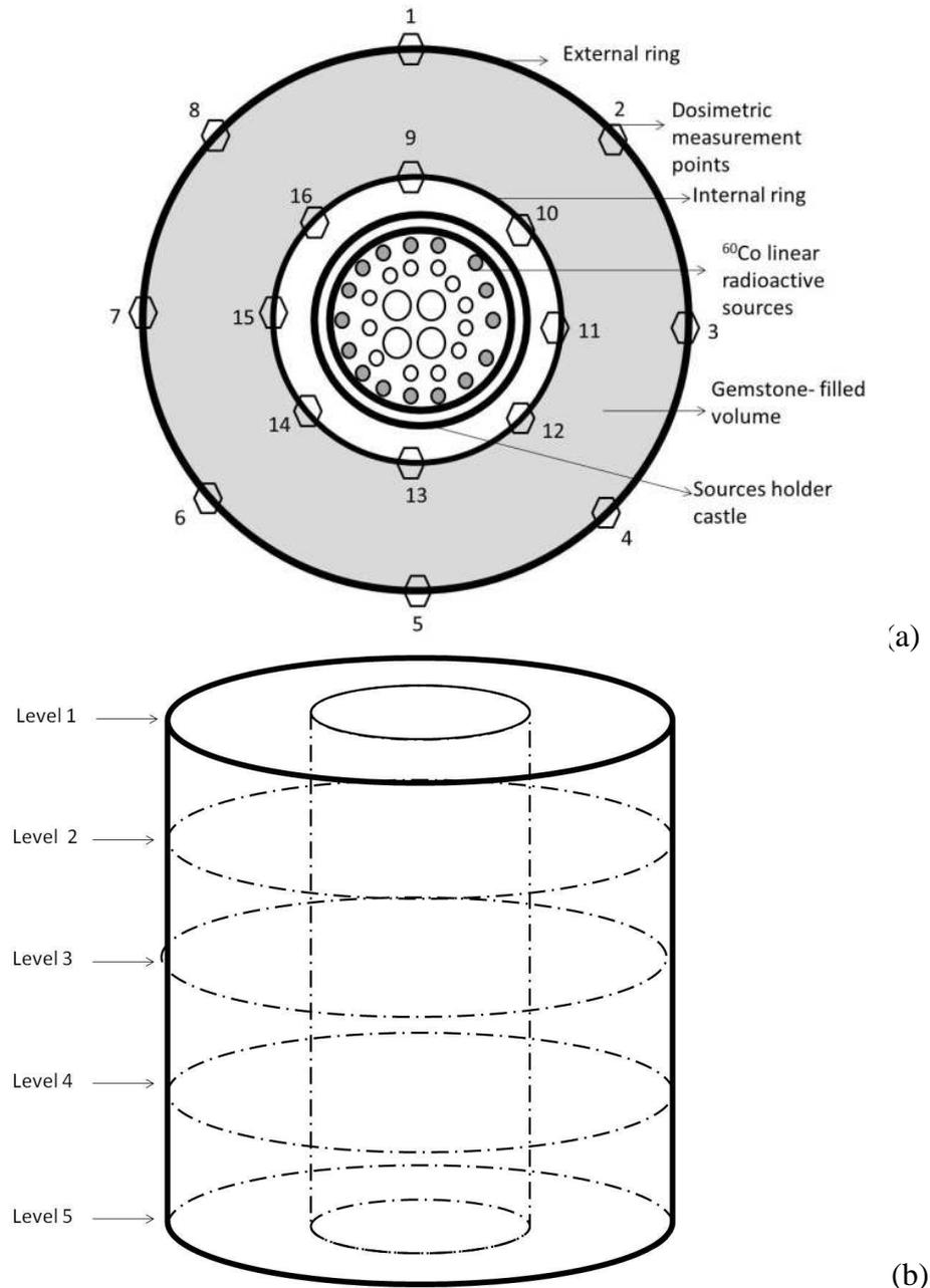
**Figure 2: (a) Cylindrical device top view and dosimetric measurement points; (b) Dosimetric measurement levels**
