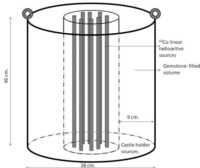
**Figure 1: Schematic view of the hollow cylindrical device.**
