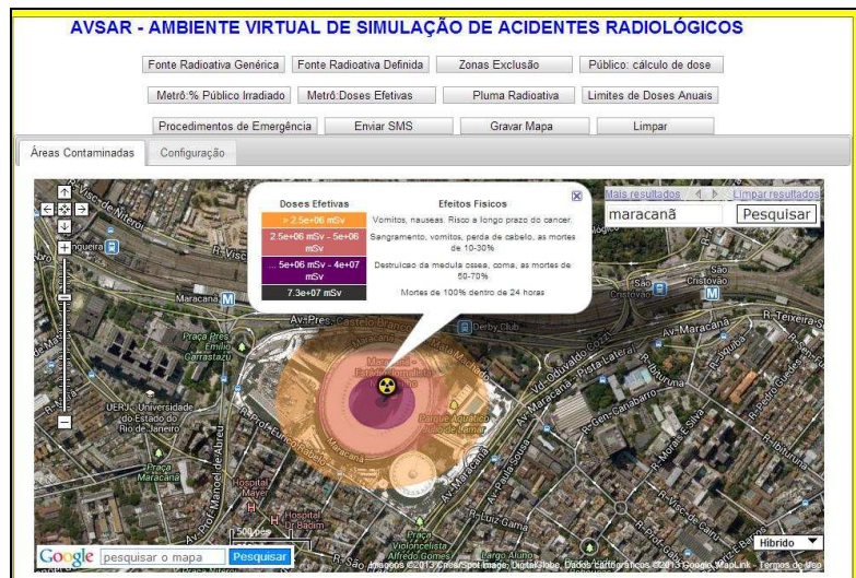
Figure 3: AVSAR - location of the radioactive source
