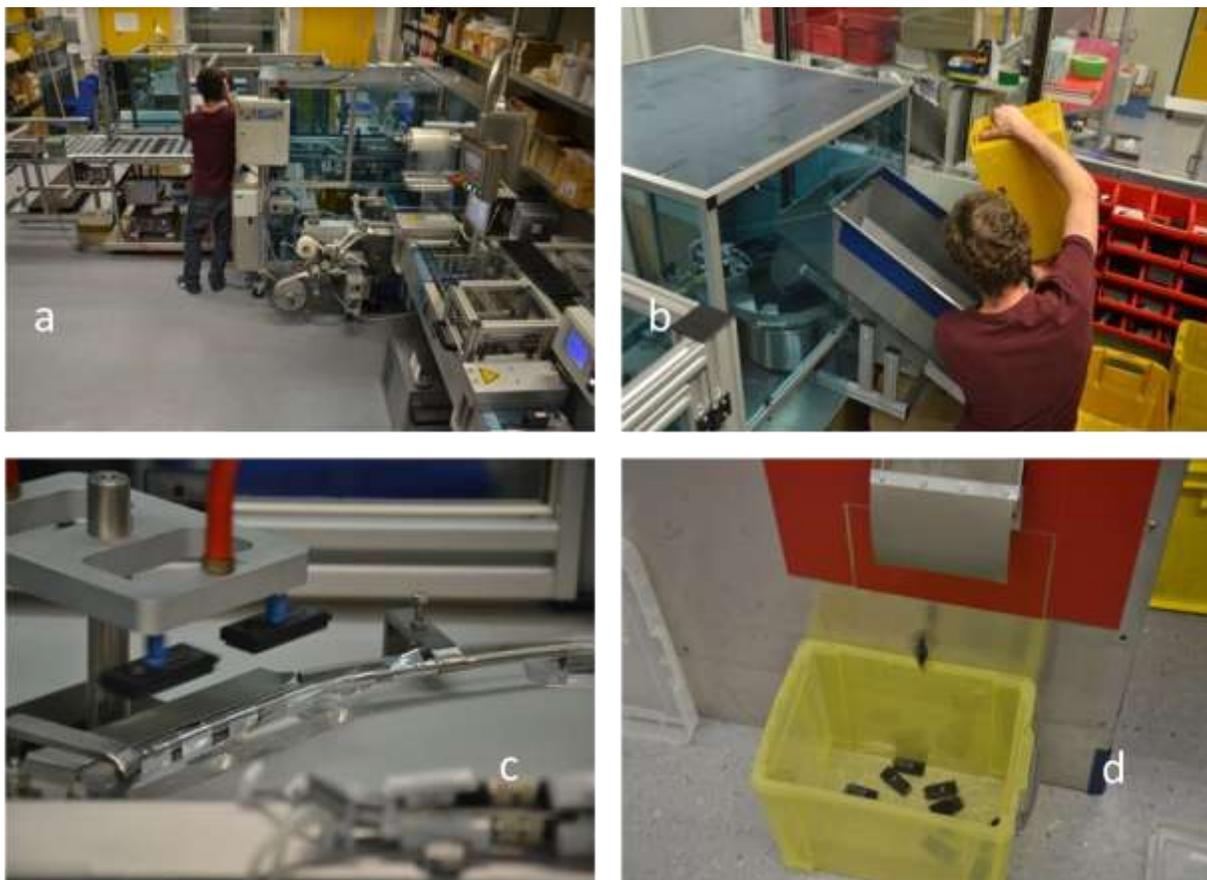
Figure 8: unpacking; a: overview; b: filling; c, d: unpacked dosimeters
