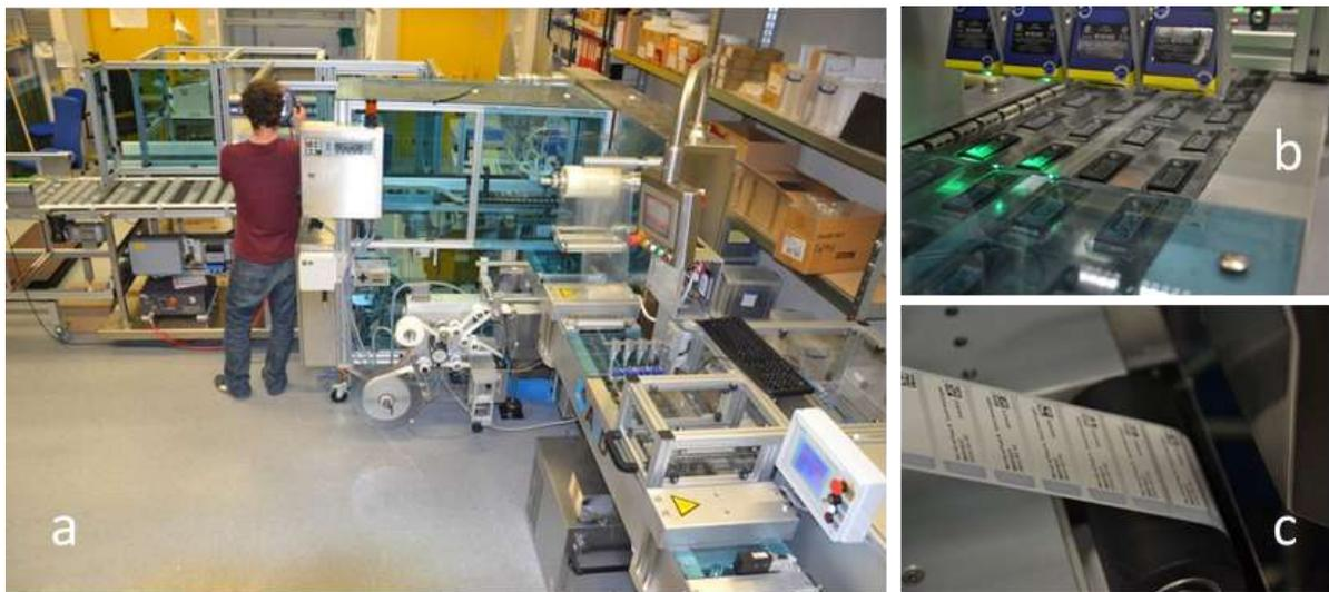
Figure 5: packing; a: overview; b: blister package; c: printing the labels
