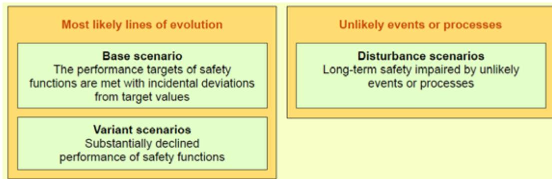
The repository system is designed in such a way that each component of the engineered barrier system (EBS) should, for most likely lines of evolution and in the absence of incidental deviations, meet the safety functions and performance targets assigned to it, and the host rock should conform to its target properties. In this case, the copper-iron canisters remain intact for the whole assessment time frame and there is no release of radionuclides.
