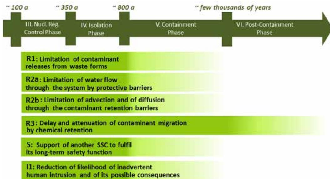
**Figure 3: Principle for the development of the safety concept**
