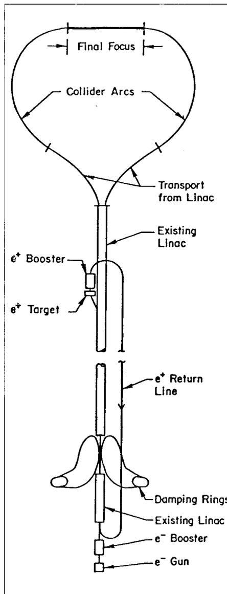
*Schematic of the Stanford Linear Collider, SLC. The upgraded electron linac of the Stanford Linear Accelerator Centre will produce positron beams which will be brought back for acceleration through the linac. Pulses of electrons and positrons will be moulded to high quality in the damping rings, accelerated along the linac to 50 GeV, sent through opposing arcs and collided. The construction and commissioning schedule aims for colliding beams in February 1987.*
