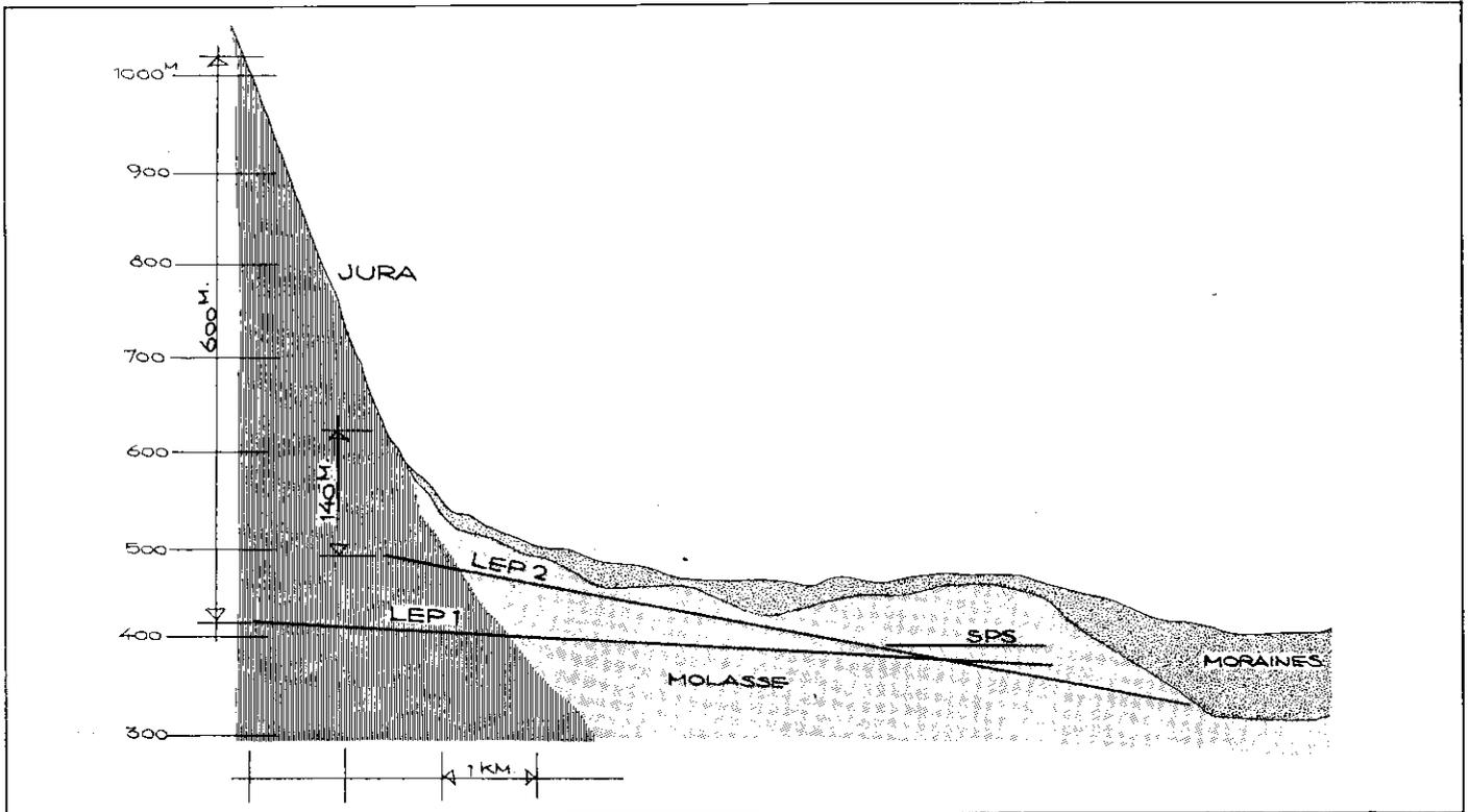
good to excavate using roadheaders and boring machines. Its characteristics were well charted at CERN after experience in building the 7 kilometre SPS Super Proton Synchrotron ring in the early seventies.
