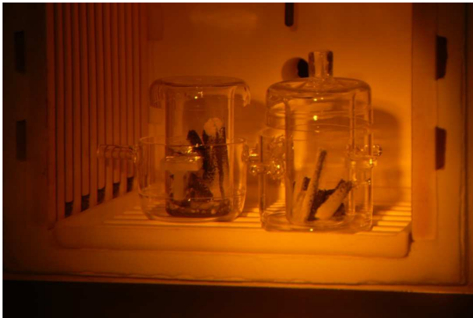
Figure 3: Graphite holder pieces following first burn step (136 hrs @ 750°C)
