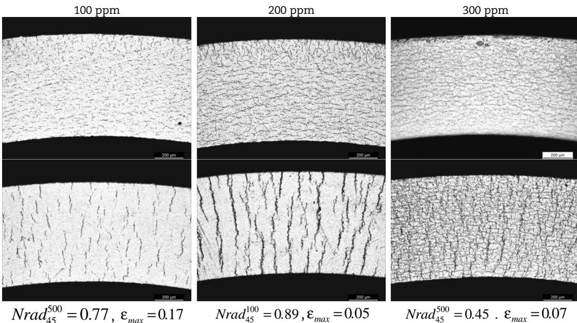
There is no agreed definition on hydride re-orientation. We consider hydrides that have an orientation larger than  $45^\circ$  from the circumferential direction as re-oriented. The re-orientation is then defined by the total length of radial hydrides divided by the length of all hydrides ( $Nrad_{45} = \sum a_i(\varphi > 45^\circ) / \sum a_i$ ). The re-orientation and other hydride parameters are derived from the image processed micrographs.
