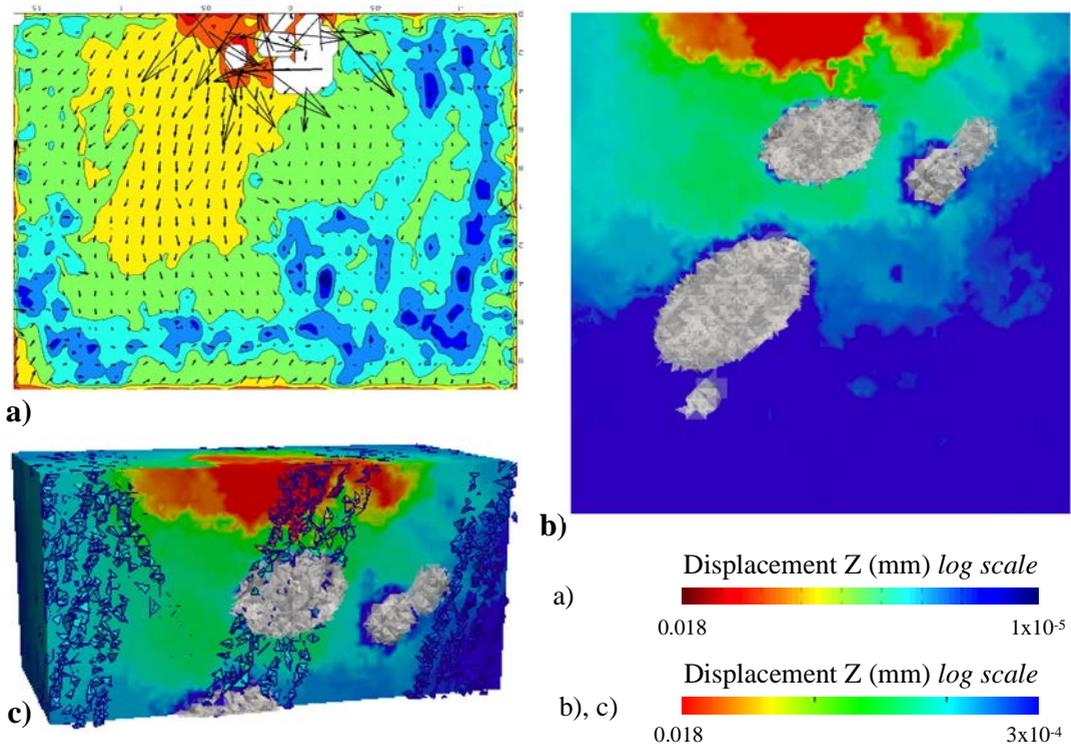
Further comparison is made using the compressive displacements and strains along the z-axis under the indentation (i.e. at  $x=1.5$  mm and  $y=1.5$  mm), which are shown in Figures 6 and 7 together with quarter slices of the CAFE numerical simulation in which the macro-pores are shown and the FEM that describes the continuum. As the CAFE
