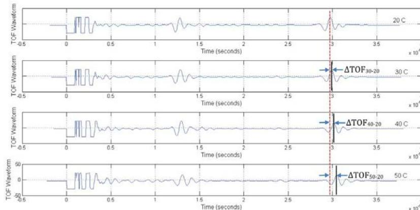
Given the measurements of the time of flight, the speed of sound in each segment between two consecutive backscatterers inside the sample,  $\text{SOS}_i$ , is calculated at each temperature using the following equation:
