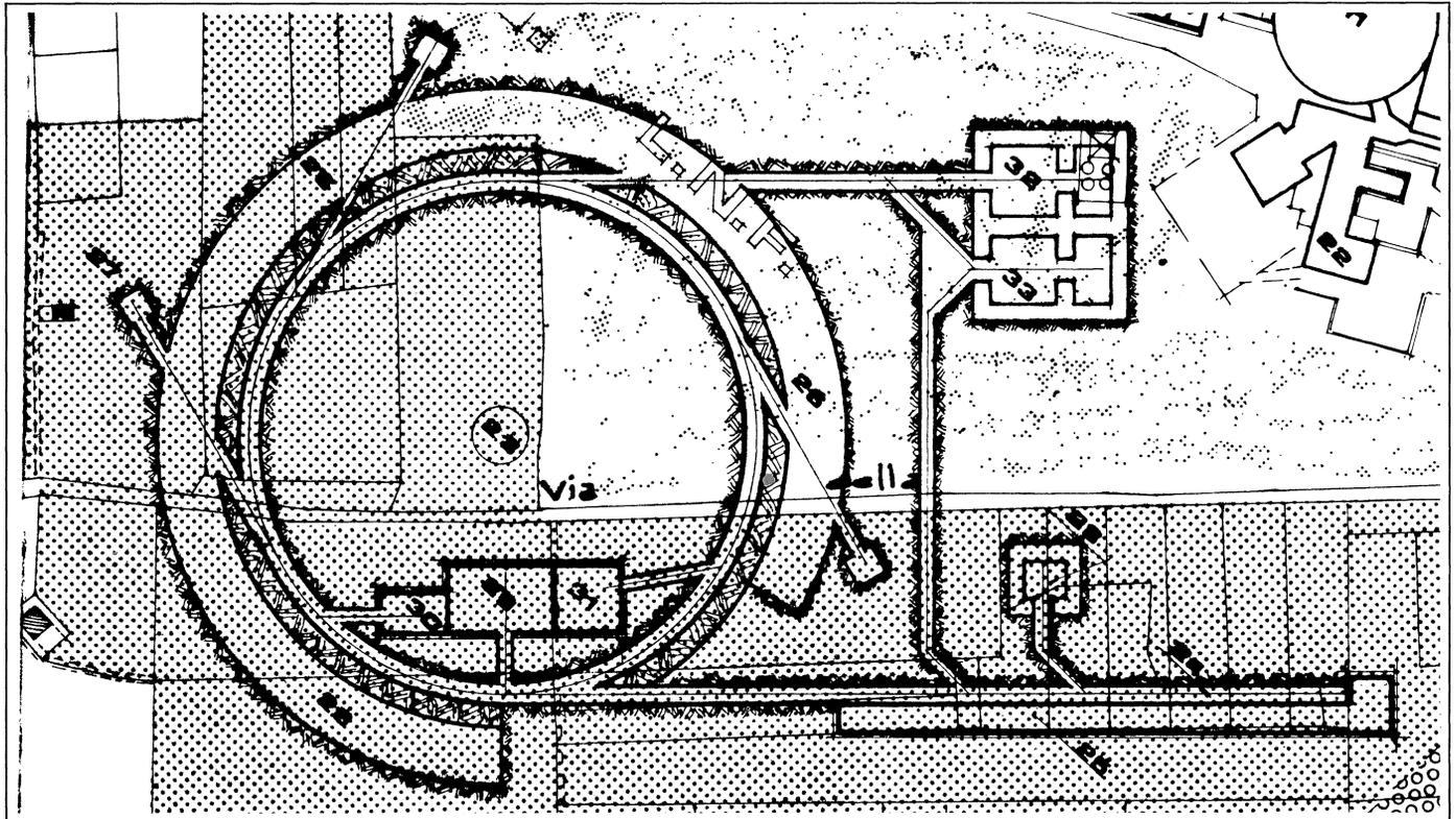
optimize both physics (in particular as far as energy was concerned) and machine requirements, a completely new electron machine was proposed, with a 1.1 GeV electron linac and a long (460 m circumference) stretcher ring. (The suffix 3 after ALFA indicates the three scientific fields covered by the new facility, rather than the number of revisions of the proposal.)
