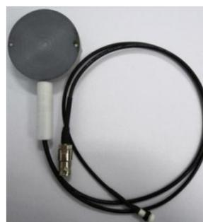
**Figure 1:** New ionization chamber developed at IPEN.
