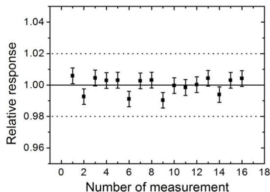
**Figure 4:** Medium-term stability of the new ionization chamber. The dashed lines represent the recommended limits of 2% (IEC (1997)).
