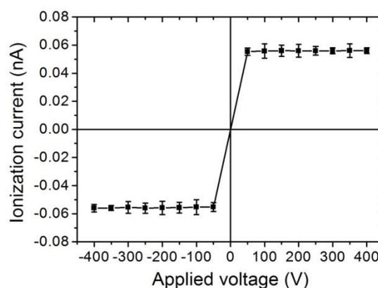
**Figure 5:** Saturation curve obtained with the RQR 5 radiation quality for the ionization chamber.
