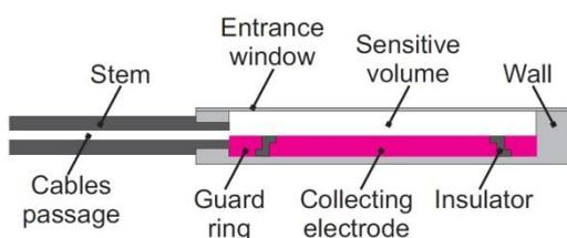
**Figure 2:** Scheme of the plane-parallel ionization chamber developed at IPEN and characterized in this work.
