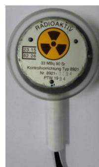
**Figure 3:** Special PMMA support and radioactive check source positioned on the ionization chamber during its stability tests.
