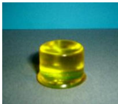
Figure 1 Acrylamide cylindrical source polymerized by high gamma dose irradiation.
