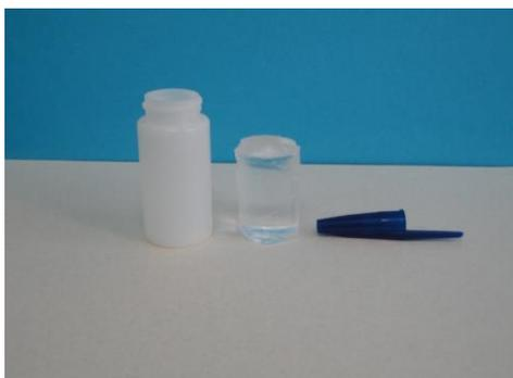
Figure 2 Plastic container and the cylindrical acrylamide/bis-acrylamide polymerized resin.
