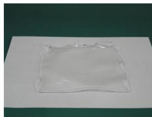
Figure 4: The flat acrylamide/bis-acrylamide polymerized resin.
