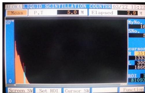
**Figure 3:** Beta spectrometry results of <sup>177</sup>Lu
