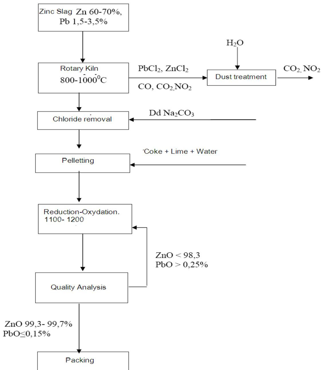
**Figure 5:** Technology schema for high quality zinc oxide(99.5%) production line.
