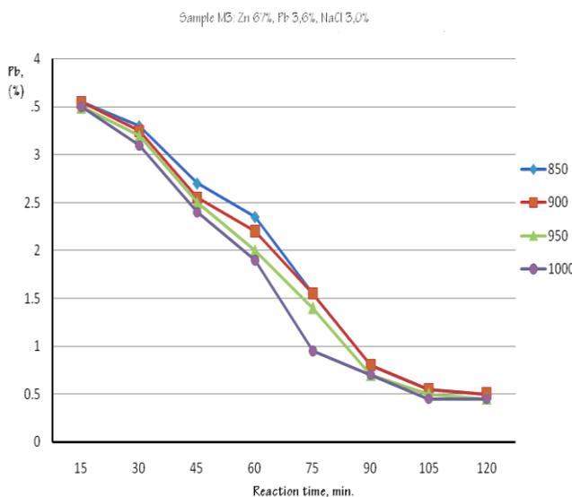
**Figure 2:** Lead removal test (Sample tested No.3).
