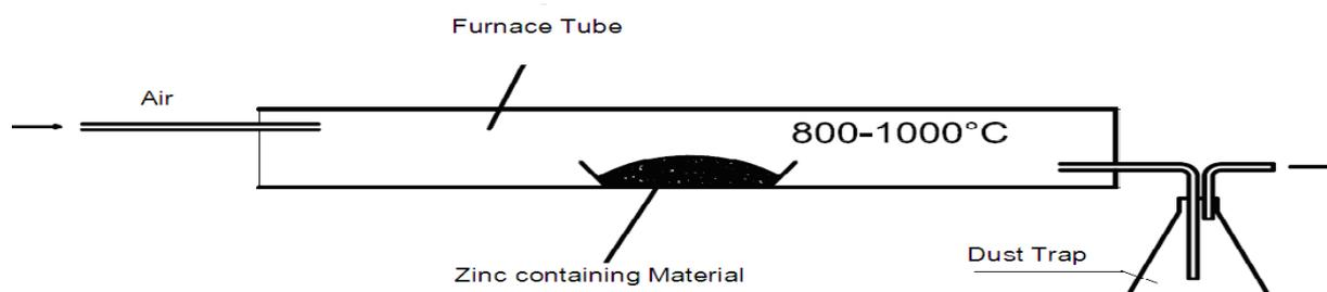
**Figure 1:** Schema of Lead removal experiment.
