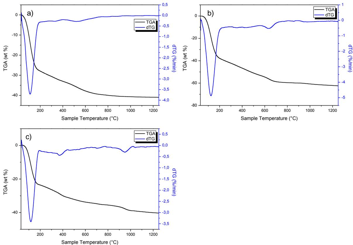
Figure 5 - TGA and dTG of the samples containing a) 0.5g ZnSeO<sub>3</sub>, b) 2.0g ZnSeO<sub>3</sub>, c) 0.5g Na<sub>2</sub>SeO<sub>3</sub>.
