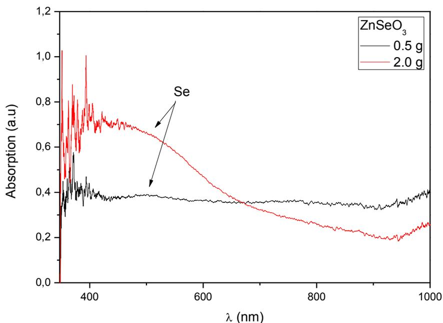
**Figure 4 - Optical absorption spectrum for samples containing ZnSeO<sub>3</sub>.**
