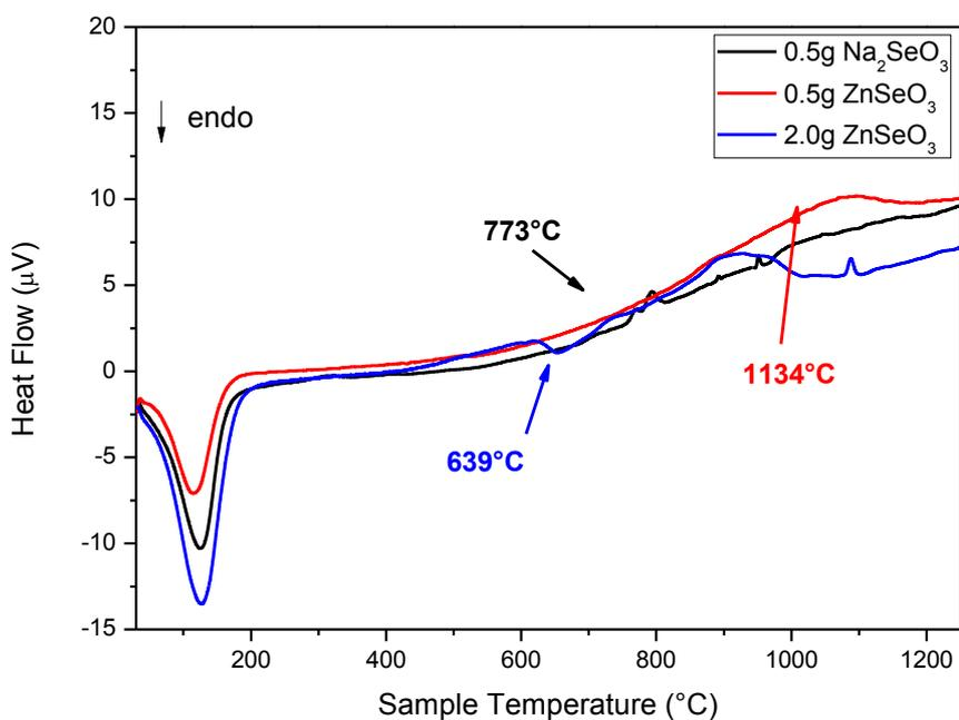
Figure 6 - DSC of the samples containing selenium precursors.
