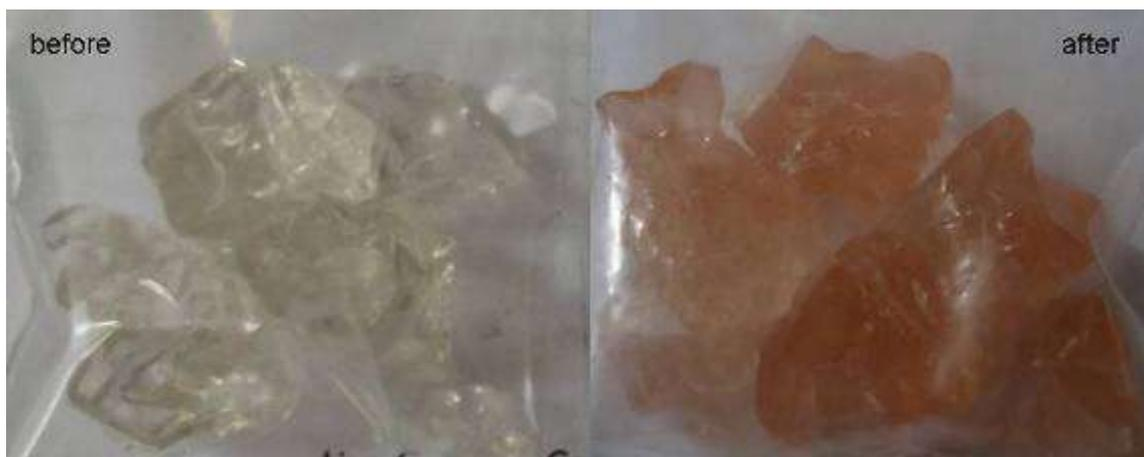
Figure 7 - Coloration changing of sample containing 2.0g ZnSeO<sub>3</sub>.
