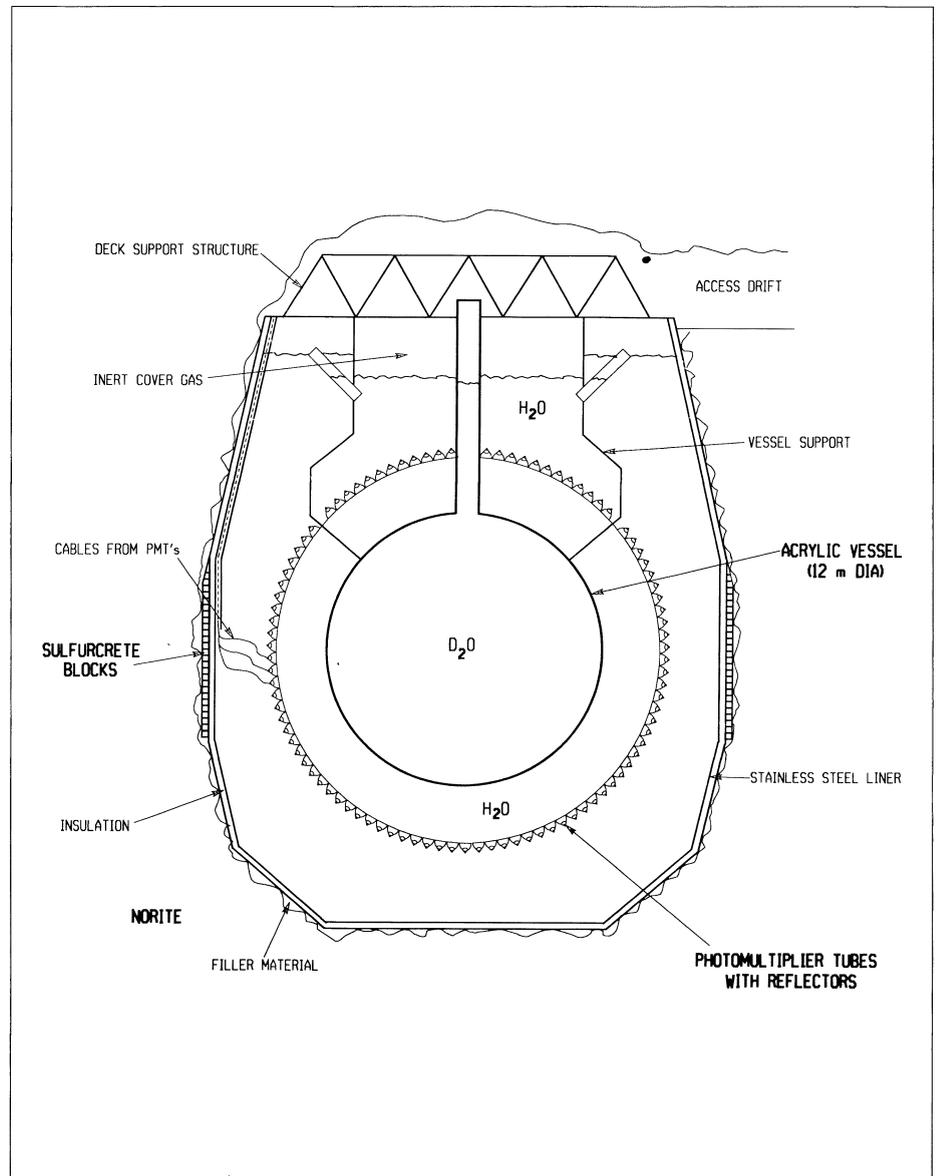
*Design for the new Sudbury Neutrino Observatory to be built 2000 metres underground in a Canadian nickel mine, showing the inner heavy water target vessel surrounded by the ordinary water vessel and banks of photomultipliers.*
