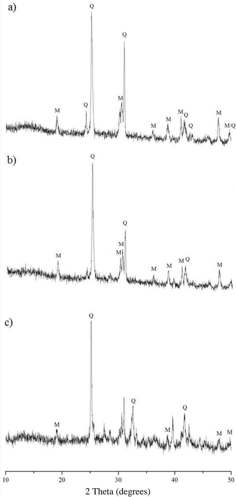
Figure 4: XRD patterns of sintered samples. (a) 7, (b) 6 (c) 3, with 14, 20 and 40% residue.
