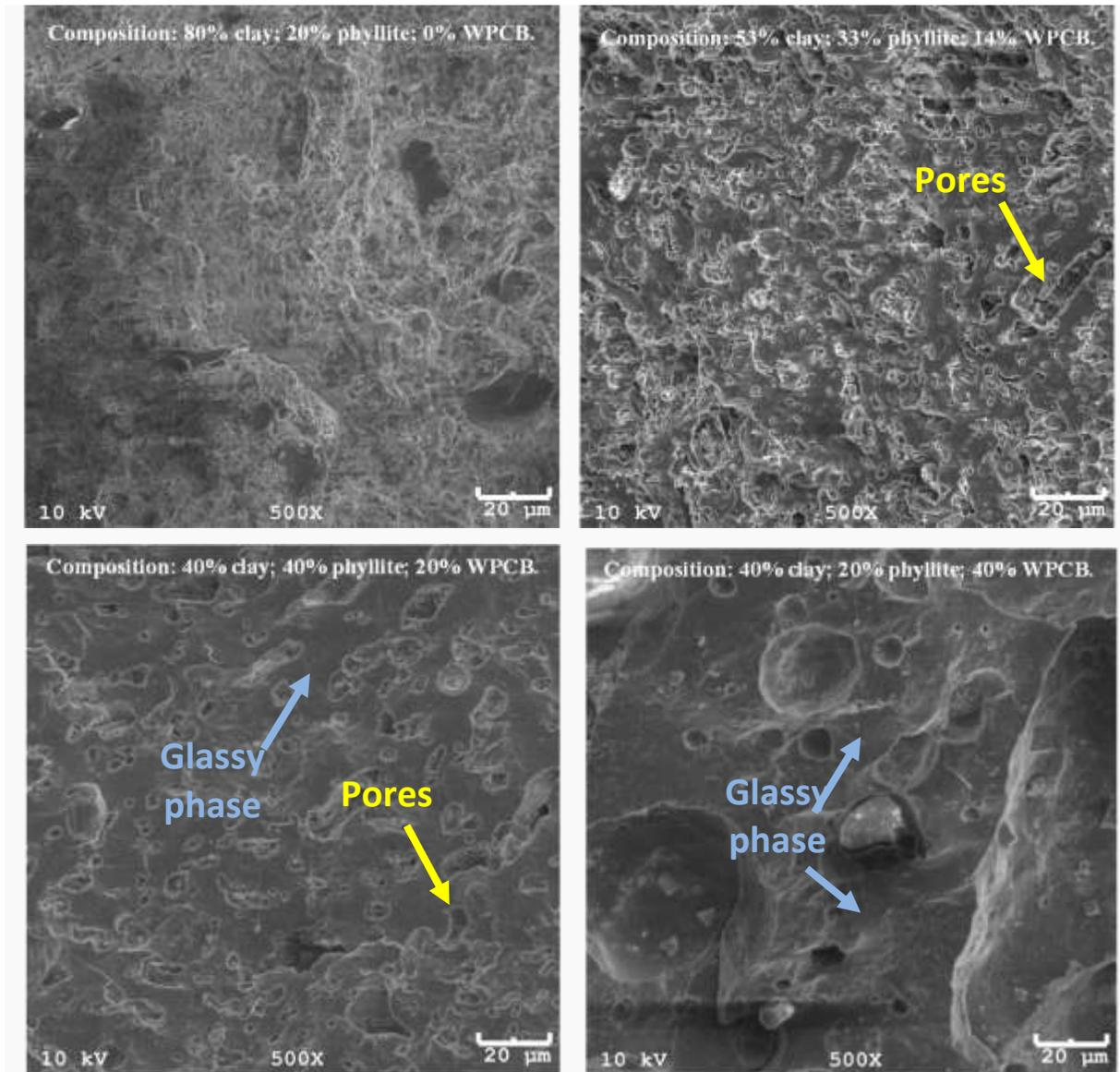
Figure 3: SEM micrographs of fractured samples containing (a) 0%; (b) 14%; (c) 20% e 40% WPCB.
