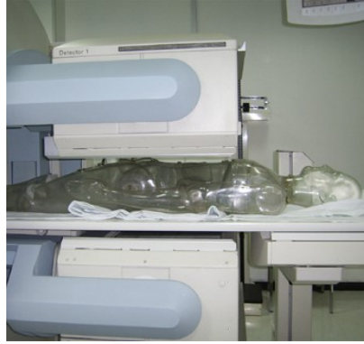
FIG.1. Water filled anthropomorphic phantom being scanned with the dual-head gamma camera.
