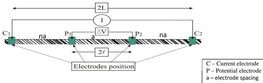
Figure 3: Schlumberger's electrode array
