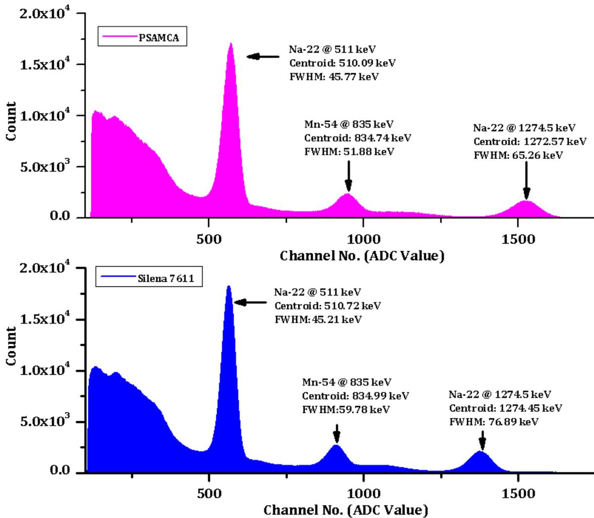
**Figure 9:** Spectral distribution of Na-22 and Mn-54 obtained with PSAMCA and Silena 7611 spectroscopy amplifier. The peaks information was extracted from a calibrated GammaVision 7 ROI file.
