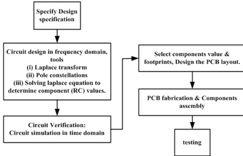
**Figure 1:** Flowchart describing the design procedure for development of the PSAMCA.
