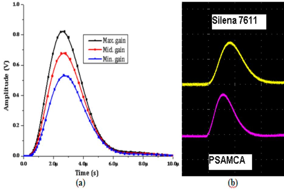
**Figure 6:** Response of the PSAMCA, (a) time domain simulation for various attainable gain at 50 mV pulser input signal and (b) oscilloscope capture of PSAMCA (pink trace) and commercial spectroscopy amplifier Silena 7611 (yellow trace) outputs, both vertical and horizontal axis scale at 200 mV/div and 5  $\mu$ s/div.
