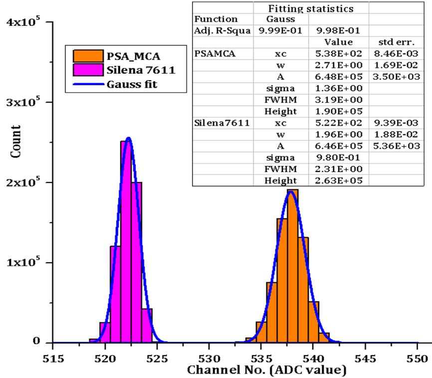
**Figure 8:** Spectral distribution of 50mV pulser signal obtained with PSAMCA and Silena 7611 spectroscopy amplifier.
