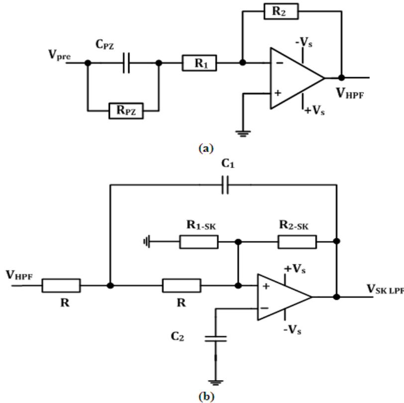
**Figure 3:** Circuits used for designing the PSAMCA, (a) 1<sup>st</sup> order high pass filter (HPF) with PZ cancellation networks and (b) 2<sup>nd</sup> order low pass filter (LPF) using Sallen-Key (SK) topology.
