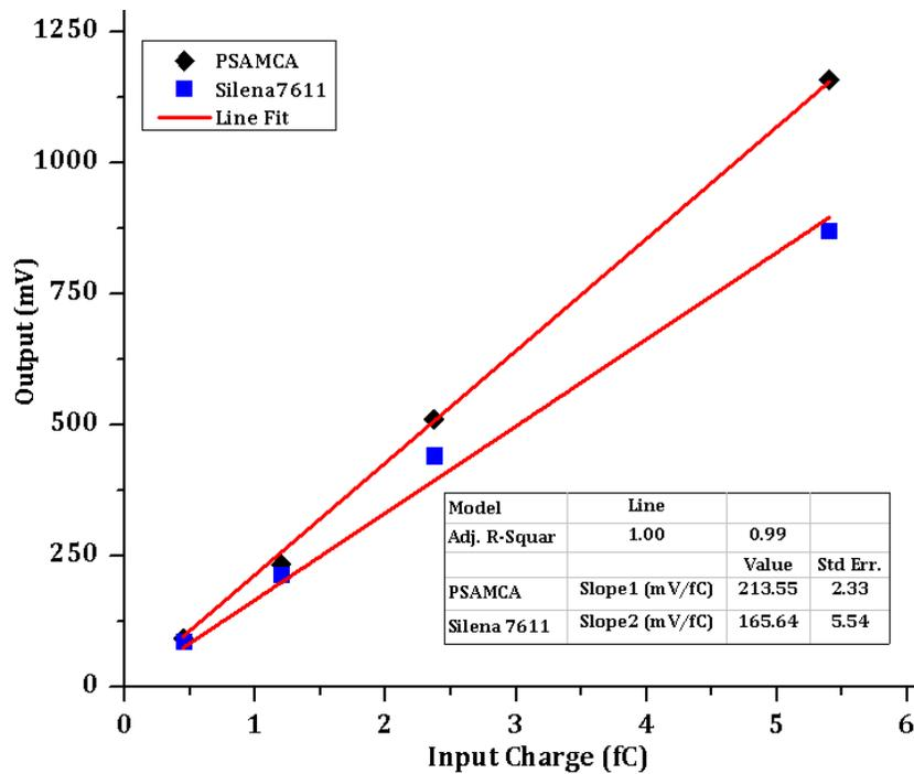
**Figure 7:** Charge sensitivity plot for both PSAMCA and Silena 7611 spectroscopy amplifier.
