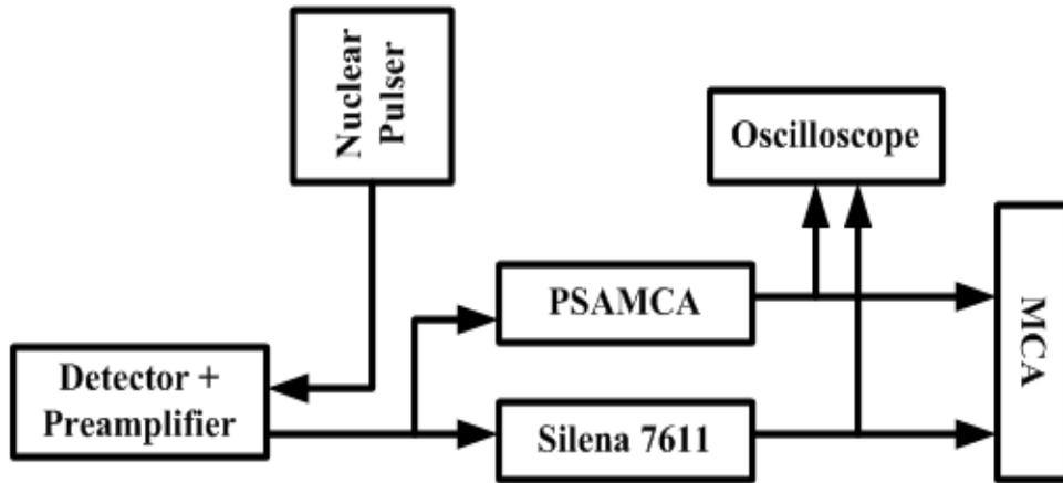
**Figure 4:** Instruments setup for measuring the PSAMCA performance.
