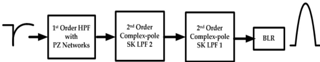
**Figure 2:** Block diagram of the PSAMCA.
