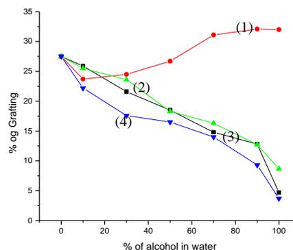
Fig.6. Effect of solvent composition on grafting. (MPTAC)=20% (w/w), total dose 2kGy under aerated condition. 1) Butanol, 2) Propanol, 3) Ethanol and 4) Methanol
