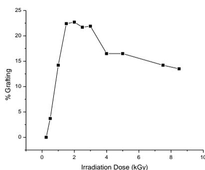
Fig. 1. Effect of irradiation dose on grafting, (MPTAC)=20% (w/w) in water, aerated solution.
