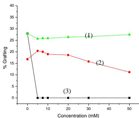
Fig.5. Effect of metal salts and acid on grafting. (MPTAC)=20% (w/w), total dose 2kGy under aerated condition. 1)  $\text{FeSO}_4 \cdot (\text{NH}_4)_2\text{SO}_4 \cdot 6\text{H}_2\text{O}$ , 2)  $\text{FeSO}_4 \cdot (\text{NH}_4)_2\text{SO}_4 \cdot 6\text{H}_2\text{O} + \text{H}_2\text{SO}_4$ , 3)  $\text{CuSO}_4 \cdot 5\text{H}_2\text{O}$ .
