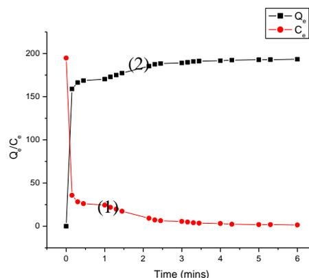
Fig.11. Adsorption equilibrium of grafted matrices versus time (G.Y. ~ 27%). [Dye] = 200ppm. 1) Q<sub>e</sub>, 2) C<sub>e</sub>.
