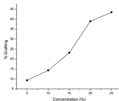
Fig. 2. Effect of monomer concentration on grafting. Total dose 5 kGy under aerated condition
