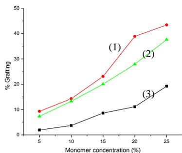
Fig. 3. Effect of ambient on grafting different concentration of monomer). Total dose 5 kGy and volume of solution 5mL. (1) N<sub>2</sub> purged, (2) Air and (3) O<sub>2</sub> saturated
