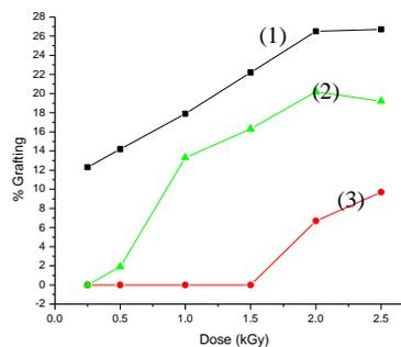
Fig. 4. Effect of ambient on grafting (different dose). Total dose 5 kGy, (MPTAC) = 20% (w/w) in water and volume of solution 5mL. (1) N<sub>2</sub> purged, (2) Air and (3) O<sub>2</sub> saturated
