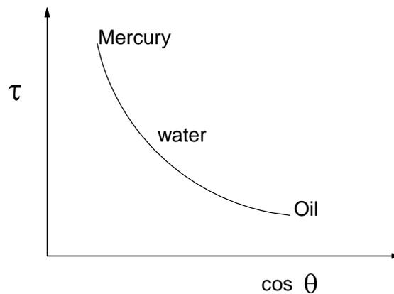
**Fig. 5:** Surface tension versus wetting ability
