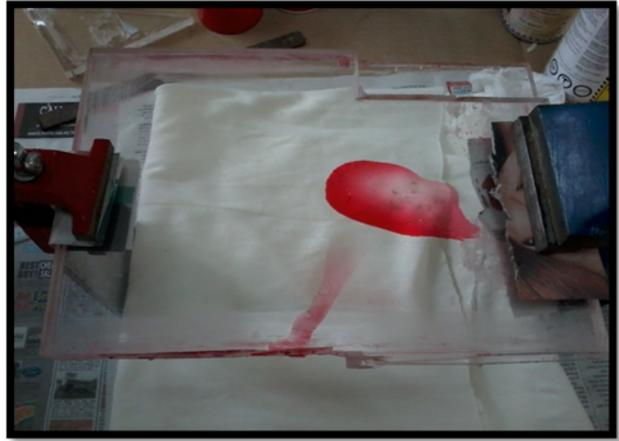
**Fig. 9:** Perspex plates clamped for penetrability test
