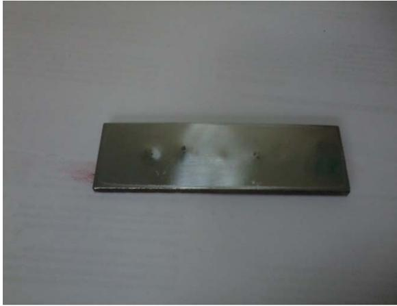
**Fig. 8:** Petrobras (Brazil) crack panel
