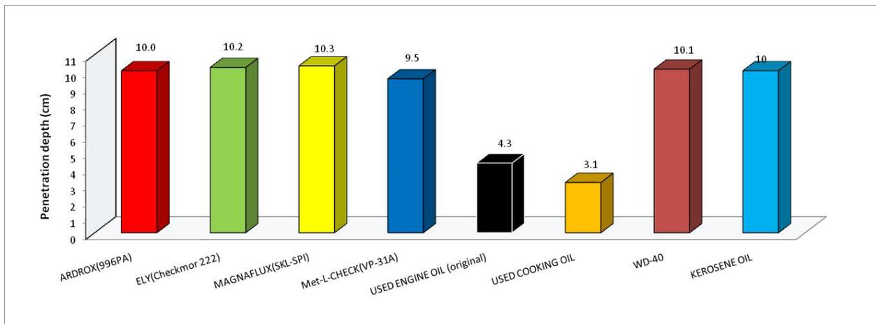
**Fig. 15: Penetration depth of different type of liquid**
