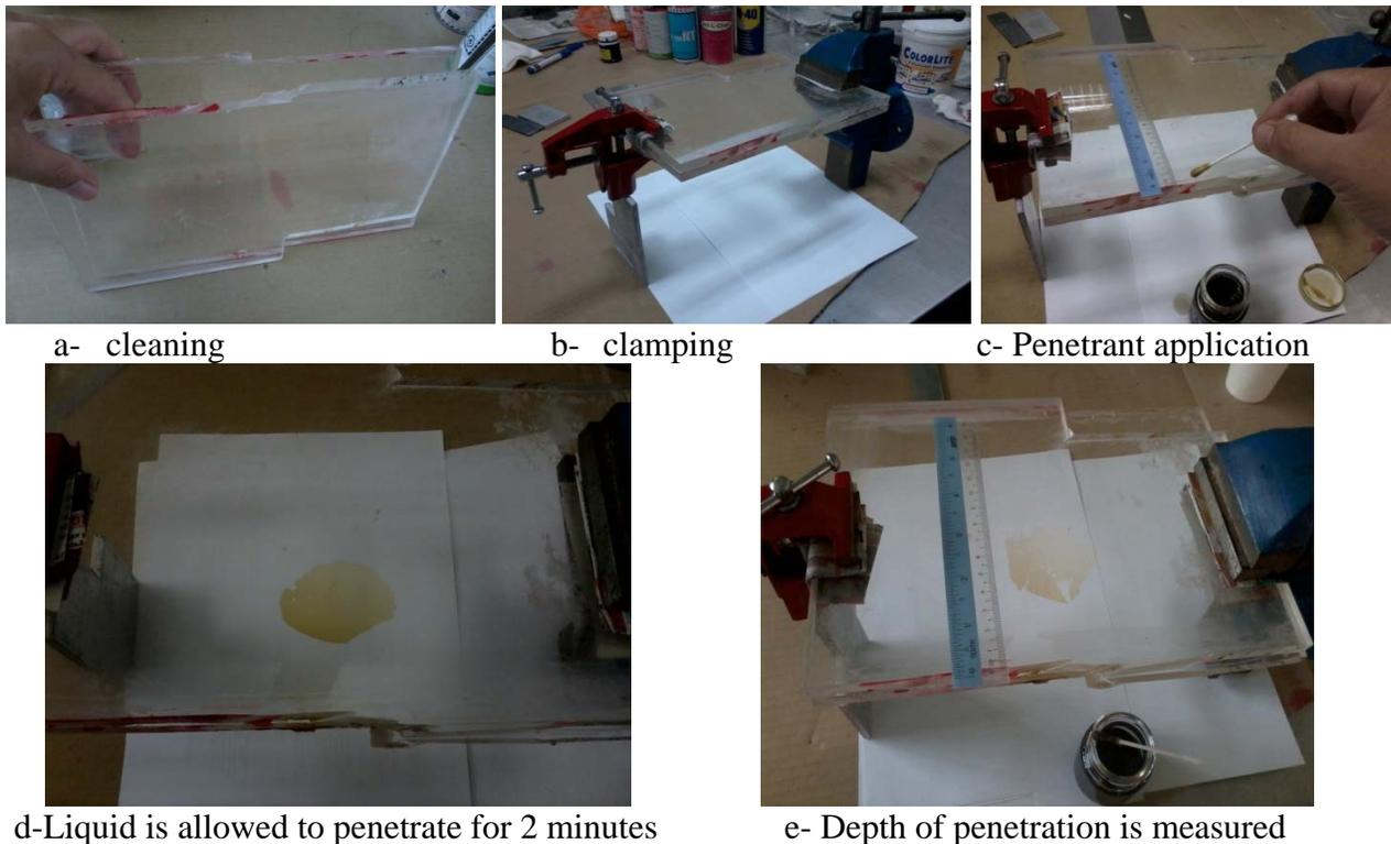
**Fig. 14:** Penetrability test
