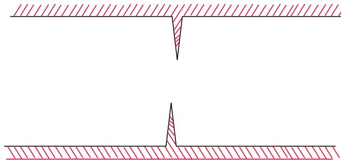
**Fig. 1:** Capillary force is not affected by gravity
