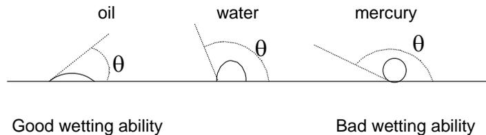
**Fig. 3:** Contact angle for different liquid
