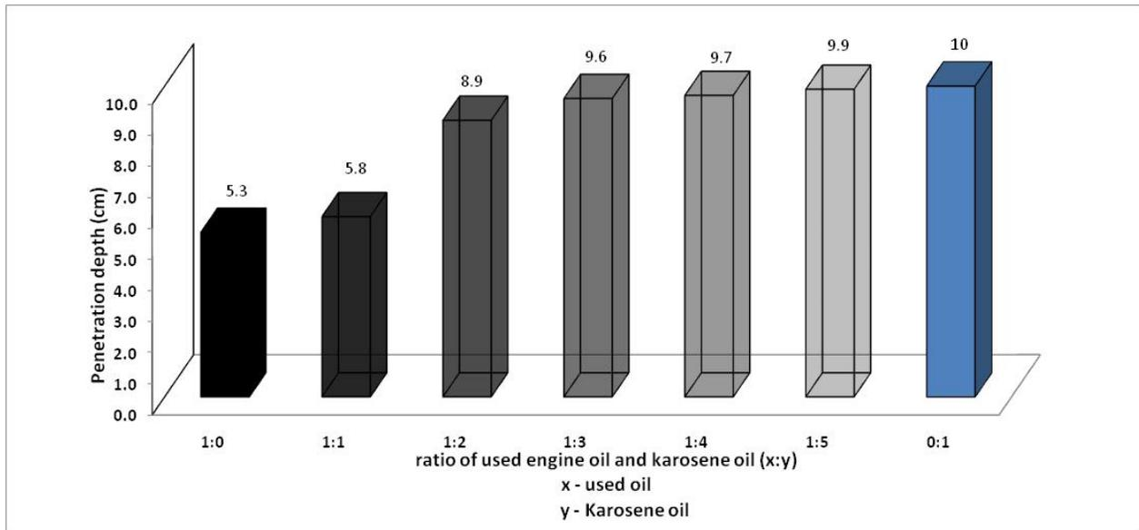
Fig. 16: Penetration depth of different dilution of engine oil/kerosene
