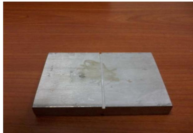
**Fig. 7:** ASME Aluminium cracked block.
