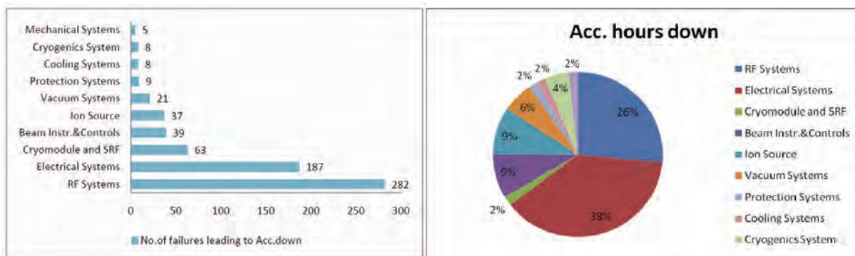
The pie chart above shows the distribution of breakdown hours by system. Accelerator trips caused by failures of components in the electrical systems represent 38% of the total accelerator downtime over the studied period. The second largest contribution is from the RF systems (26%), which are also the systems more often involved in failures leading to short accelerator trips (up to 0.2 hours).
