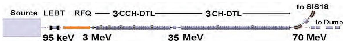
Modern H-type cavities offer highest shunt impedances of resonant structures of heavy ion linacs at low beam energies  $< 20$  MeV/u and enable the acceleration of intense proton and ion beams. One example is the interdigital H-type structure. The crossed-bar
