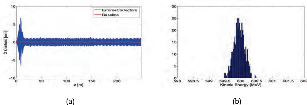
**Figure 4. Figure 5: TRACK simulations of the fault-recovery of the first cryomodule with errors and correctors**
