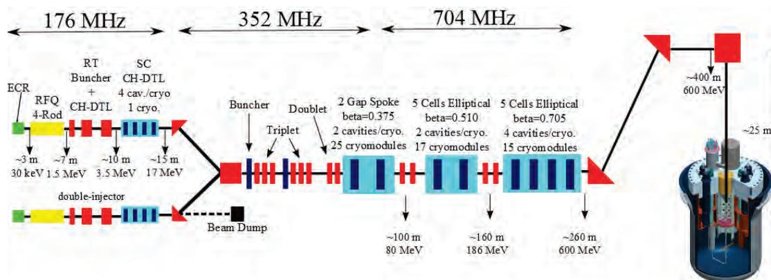
The 30 keV proton beam from the ECR source is bunched and accelerated by a 4-rod Radio-Frequency Quadrupole (RFQ) to an energy of 1.5 MeV with an average current of 4 mA. Downstream the RFQ, a buncher and 2 cooper multicell CH-DTL cavities further accelerate the beam to 3.5 MeV.
