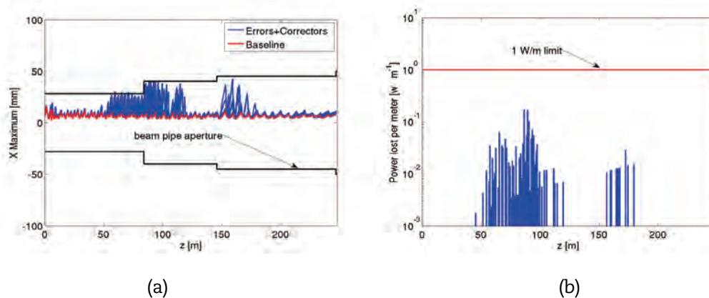
(a) Maximum horizontal beam excursion along the linac, (b) corresponding average power lost per metre along the linac.
