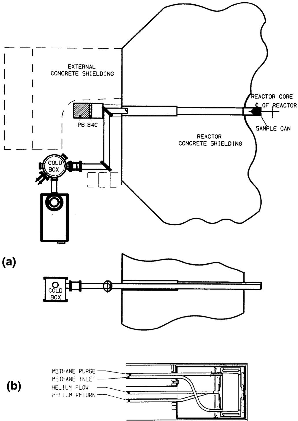
Figure 2. The CARE Reactor Test Experiment. (a) Schematic Layout of the Experiment (b) Cross Section of the Sample Can
