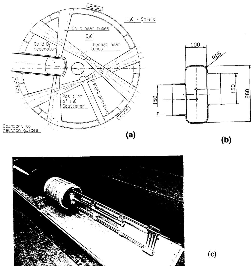
Figure 3. The SINQ D2O Moderator Tank with its T-Shaped Penetrations for Scatterer/Moderator inserts. (a) Horizontal section through the moderator tank (b) dimensions of the tubes holding the current H<sub>2</sub>O – scatterer (c) View of the current insert with H<sub>2</sub>O scatterer.
