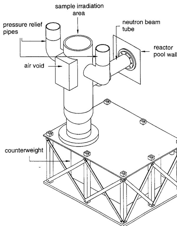
Figure 1. Moderator Test Insert Designed by ANL for the Penn State TRIGA Reactor (1 MW).
