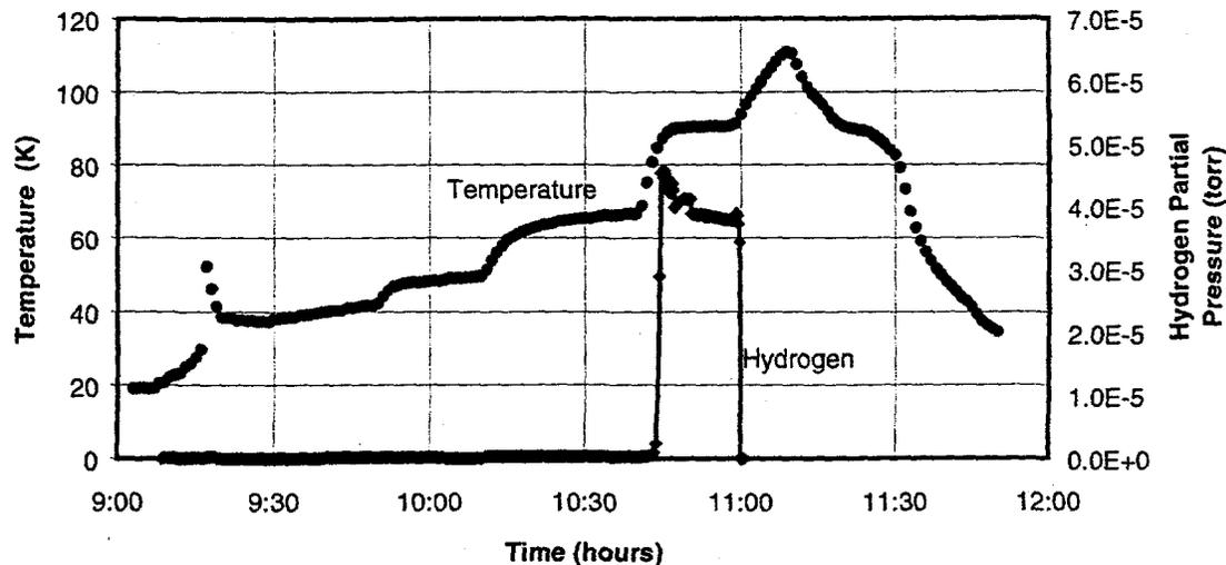
Figure 2. Hydrogen release during moderator anneal.
