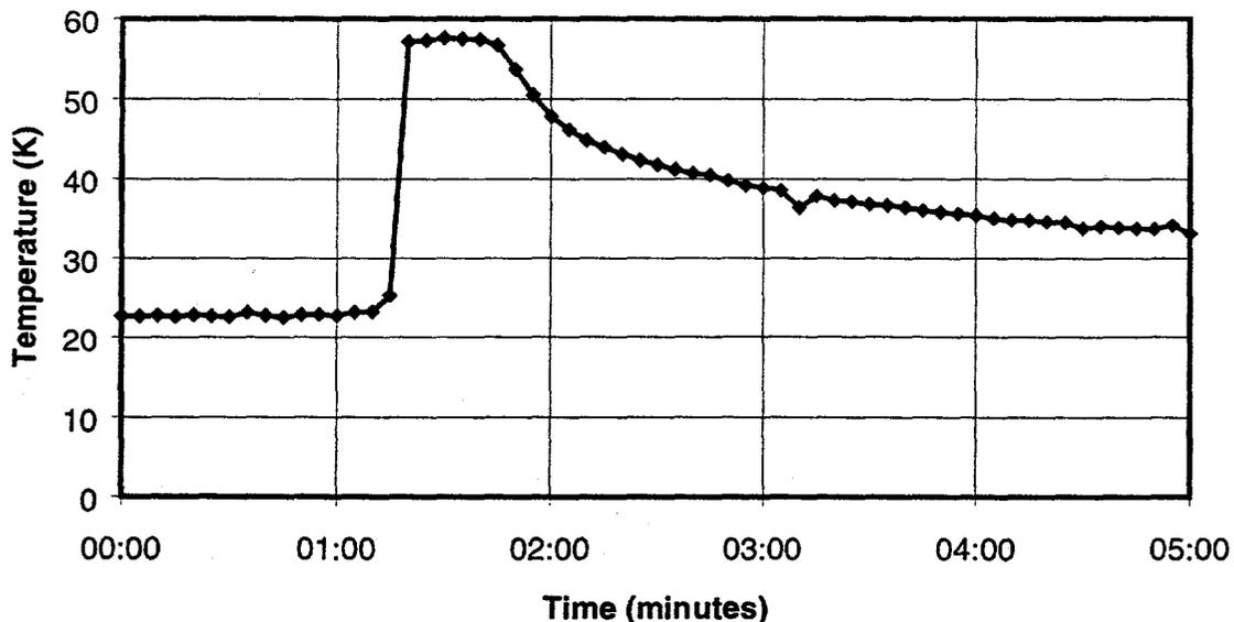
Figure 1. Stored energy release during moderator anneal.
