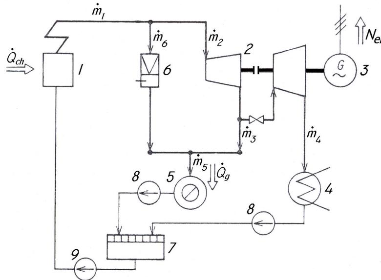
Fig.1:Scheme of thermal cycle:1-the boiler, 2-turbine, 3-electric generator,4 -condenser, 5-heat sink, 6-reduction–cooling station, 7–the condensate tank, 8-the condensate pumps, 9-feed water pump
