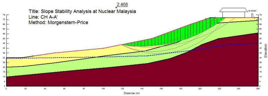
Figure 3: Stability Analysis of CH A-A'
