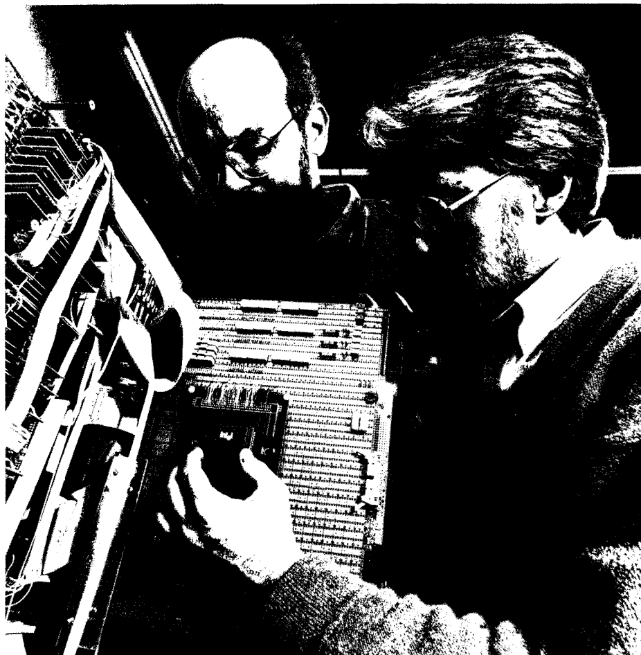
At Fermilab, Bruce Denby (right) and Clark Lindsey fit a special chip to the neural network board attached to the readout motherboard of their drift chamber. In this pioneer neural network hardware experiment, muon track angles and intercepts are calculated on-line from the chamber's analog sense wire signals. The agreement between network and offline track fitting is excellent (below).
