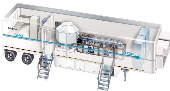
**Figure 4.** AccySys PULSAR® - 7 in a mobile configuration, mounted in a Medical Coaches 48 ft semi-trailer [2].
