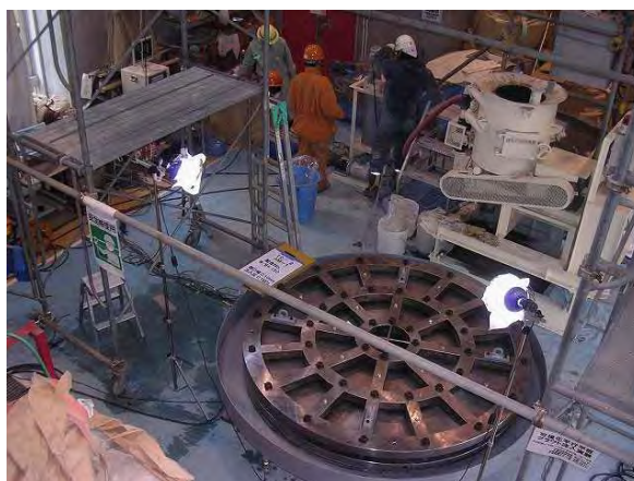
Plate 1: Overall Experimental setup. Birds-eye view of the Parallel Plate Fracture Model and Experimental System
