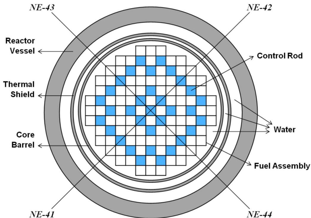
Figure 1: Reactor layout
