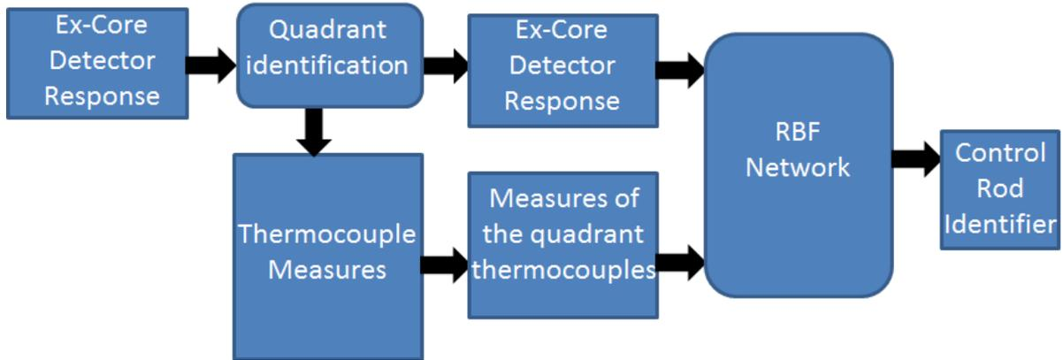
**Figure 6: Scheme for the expert system**
