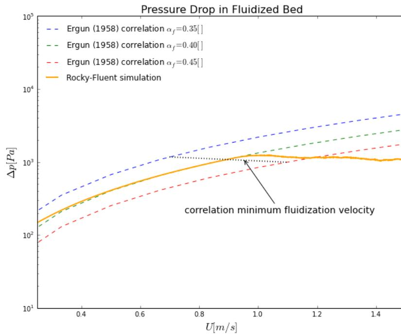
**Figure 7: Pressure drop in fluidized bed case - comparison between simulation and correlation results.**
