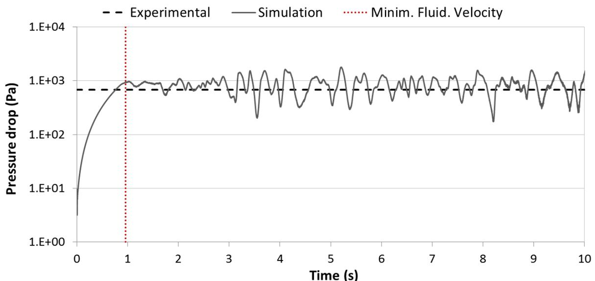
**Figure 8: Evolution of pressure drop between the two pressure intake locations - comparison between simulation and experimental results.**
