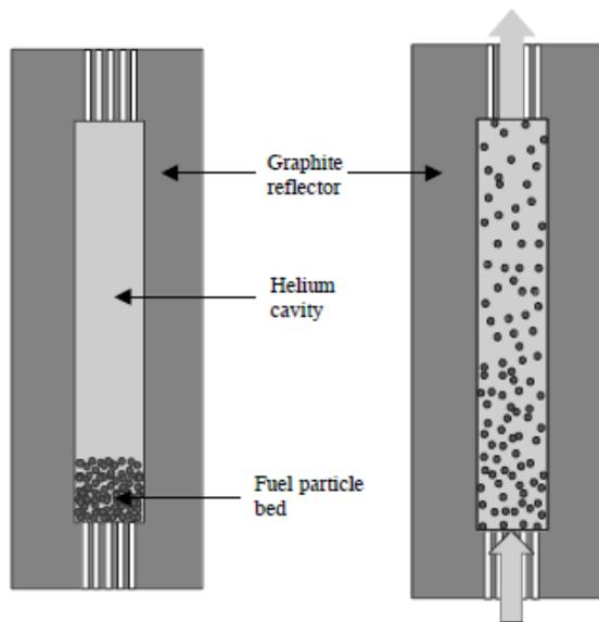
**Figure 1: Schematic view of a fluidized bed reactor at packed condition (left) and at fluidized state (right).**
