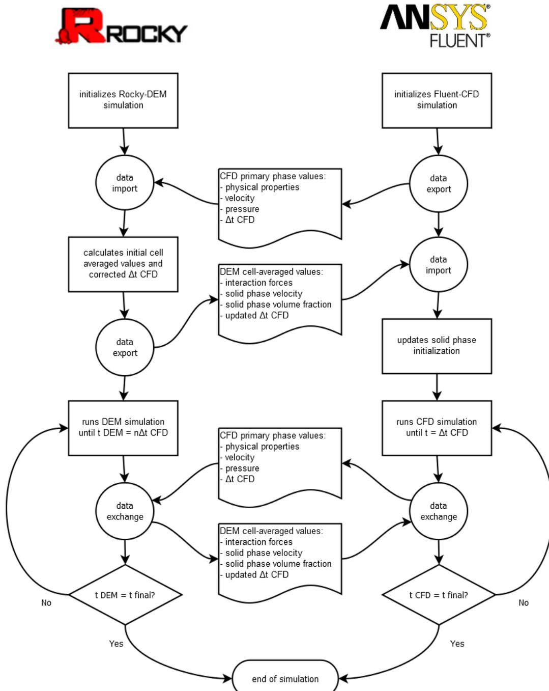
**Figure 4: Schematic algorithm of the coupling numeric between Rocky® and Fluent®.**
