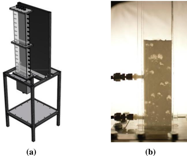
**Figure 5: (a) SSCP-I test facility and (b) Experimental facility showing pressure intakes**
