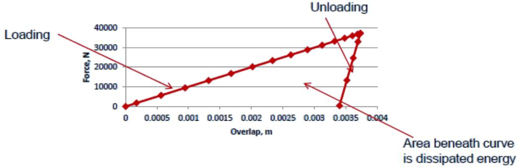
**Figure 3: Normal force from Rocky simulation at a collision of 100 mm particle on a flat plate.**
