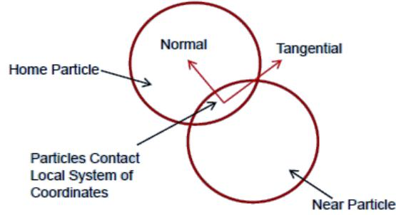
**Figure 2: Particle contact force with overlapping particles.**
