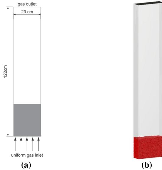
**Figure 6: (a) computational domain and fluid boundary conditions (b) initial particles bed**
