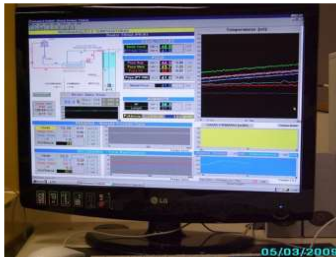
Figure 2: One of the user interface of the data acquisition system developed for IPR-R1 reactor.
