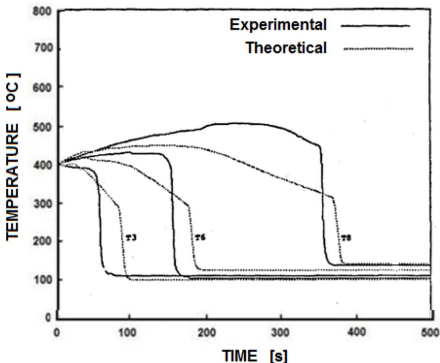
**Figure 5: Experimental and Calculated Evolution of Wall Temperature in Test 1.**
