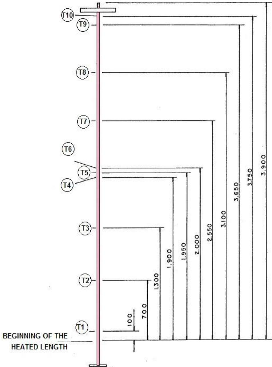
**Figure 4: Thermocouple Distribution along the Test Section**
