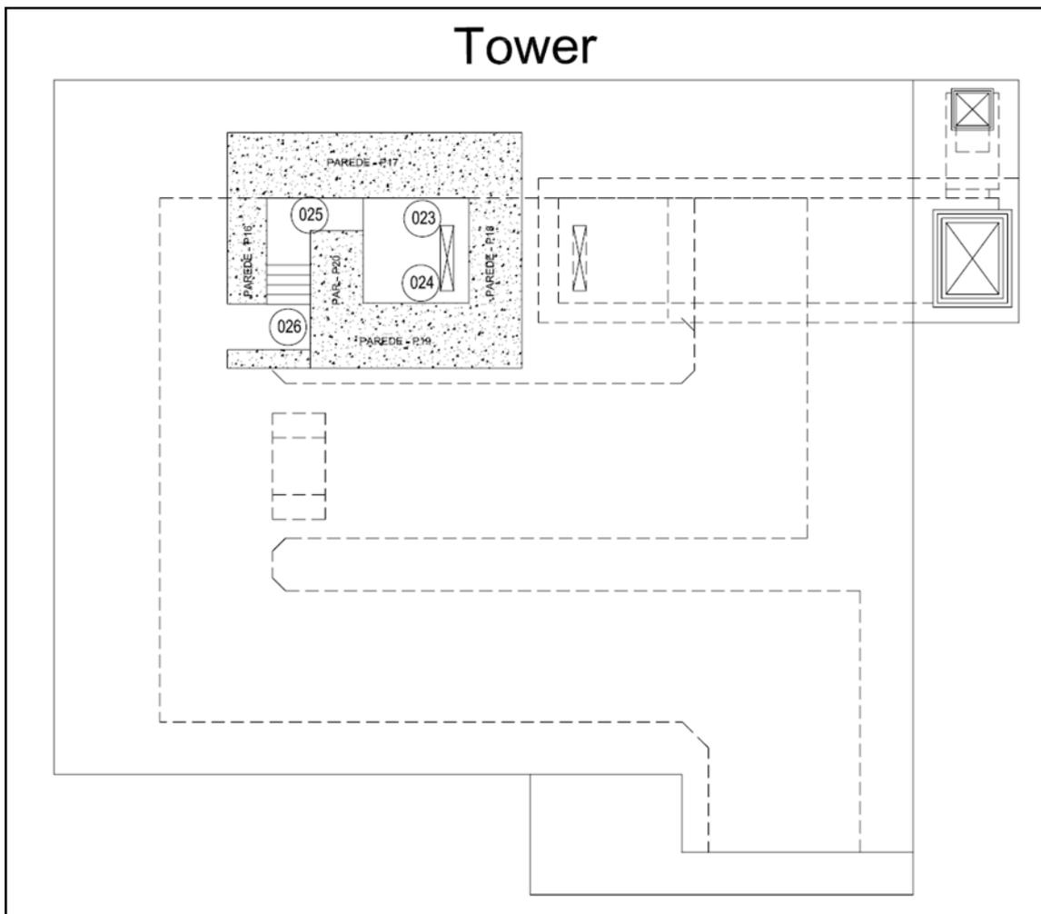
**Figure 4: Position of dosimeters in the tower of the linear accelerator (dosimeters 023 to 026).**
