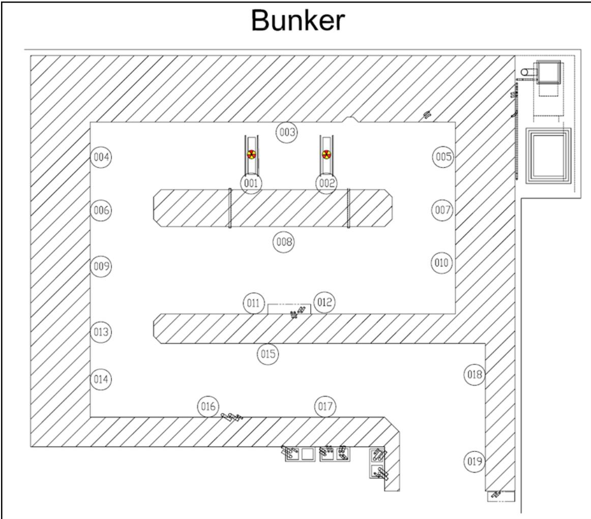
**Figure 2: Position of dosimeters inside irradiation room and near the machine of the linear accelerator (dosimeters 001 to 019).**
