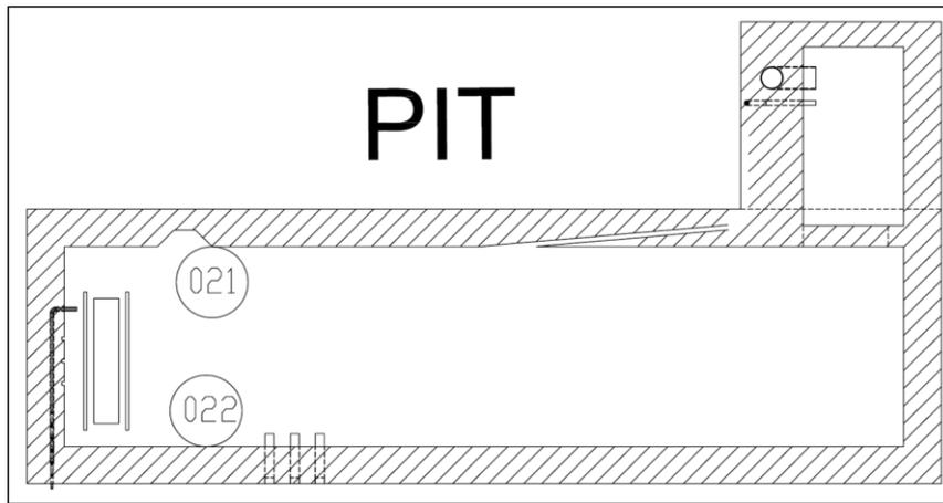
**Figure 3: Position of dosimeters in the pit of the linear accelerator (dosimeters 020 to 022).**
