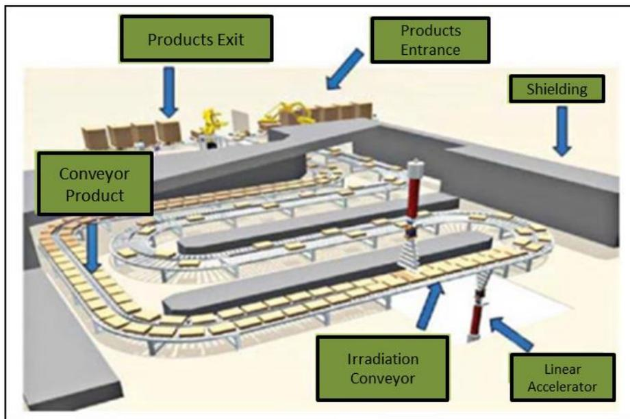
**Figure 1: Linear Accelerator - Acelétron Company.**
