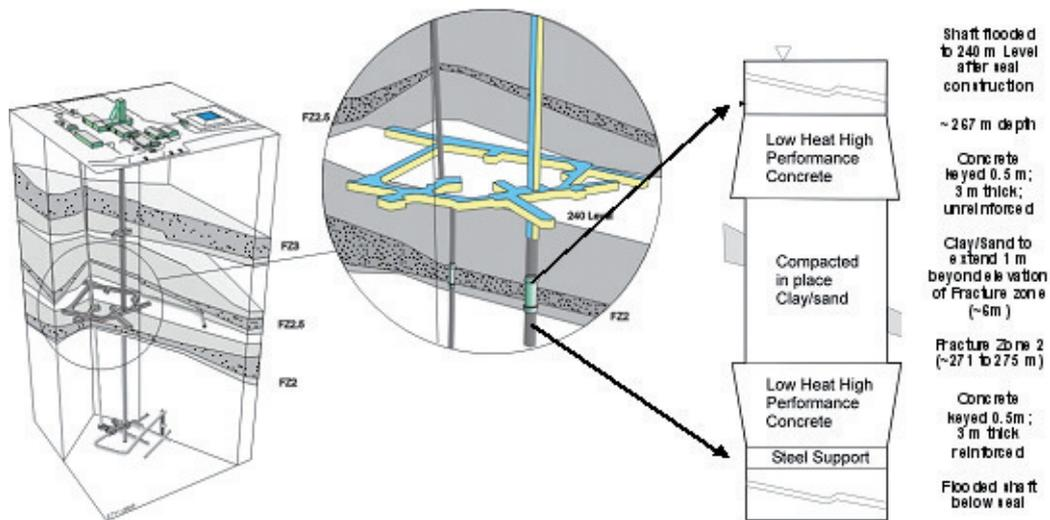
**Figure 3:** Geologic structure at URL, underground development at 240-Level and schematic showing basic layout of ESP in main shaft.
