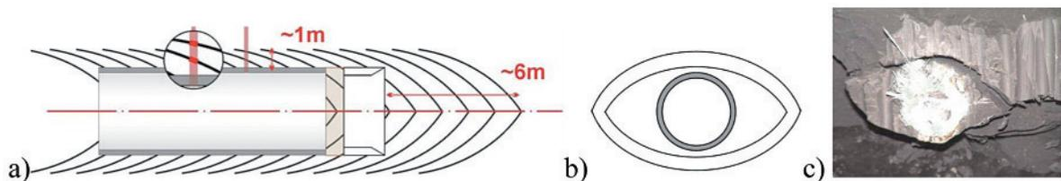
**Figure 3:** Fracture patterns in Boom Clay, a) in a vertical plane along the gallery axis, b) in a plane perpendicular to the gallery axis, c) around a small diameter injected borehole.
