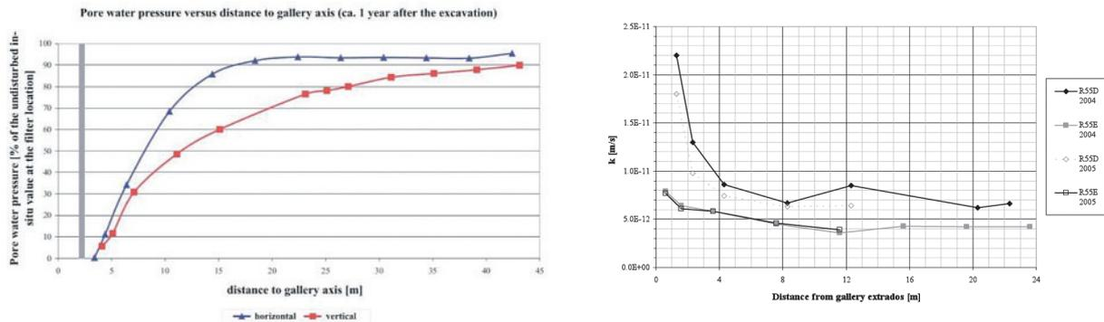
**Figure 2:** a) Horizontal and vertical radial profiles of the hydraulic perturbation caused by the excavation of the connecting gallery at Mol; b) Hydraulic conductivity measurements.
