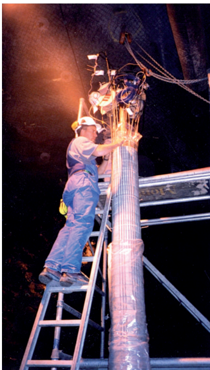
Figure 1: Installation of a test parcel (left). Measured cation exchange capacity in the bulk material from parcel A2 as a function of distance from the copper tube (upper right). Deviator stress versus strain (lower right). Red color indicate material from warm positions and blue from cold.
