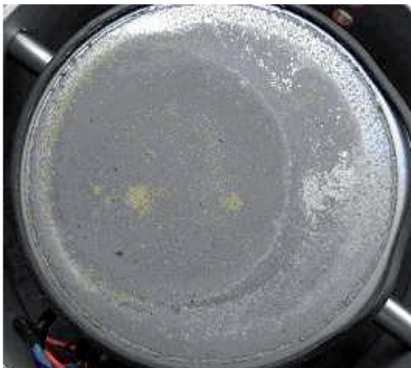
Figure 3: Carbon steel plate after experiment with ventonite Rokle at 80°C.
