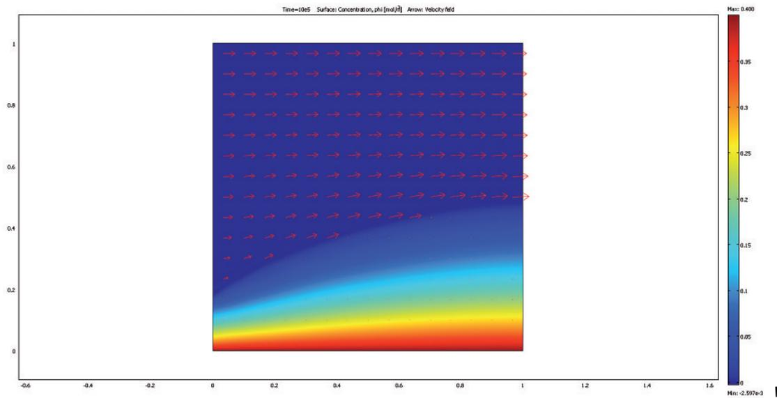
**Figure 2:** Smectite volume fraction distribution and water velocity field in the fracture.
