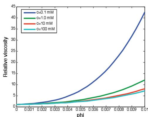
**Figure 1:** Relative viscosity as function of the smectite volume fraction for different sodium concentrations.
