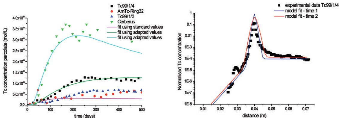
**Figure 1:** (left) Tc concentration in the percolate of four different migration experiments performed under lab (Tc99/1/4 and Tc99/1/3) or *in situ* conditions (Am-Tc-Ring32 and Cerberus). Model fits are continuous lines.
