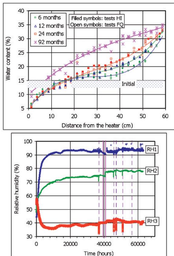
**Figure 2:** Left: Final water contents along the 60-cm long bentonite columns. Right: Evolution of relative humidity in a 40-cm long bentonite column hydrated under thermal gradient (sensor 1 placed at 30 cm from the heater, sensor 2 at 20 cm and sensor 3 at 10 cm).
