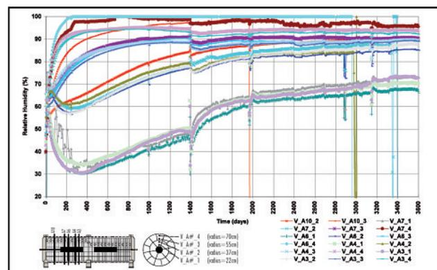
**Figure 1:** Left: Evolution of the relative humidity of the bentonite at 3.5 cm from the heater and at approximately the same distance from the gallery wall (54 cm) in a section not affected by the heater of the FEBEX *in situ* test. Right: Evolution of the relative humidity of the bentonite in various locations of the FEBEX mock-up test.
