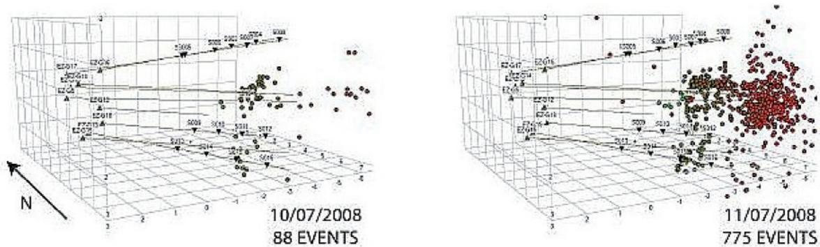
**Figure 2:** Acoustic emissions located inside the rock mass at two different dates: in green, the emissions probably indicate a fault reactivated by the excavation process.
