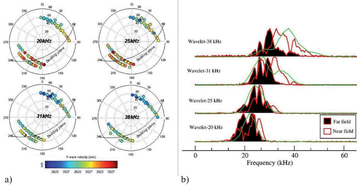
**Figure 1:** (a) Stereograms of the P-wave velocities, suggesting an anisotropic properties of the rock mass, derived from far field tomography at different wavelet frequencies; (b) Signal recomposition showing frequency resonances increasing with the distance to the source.
