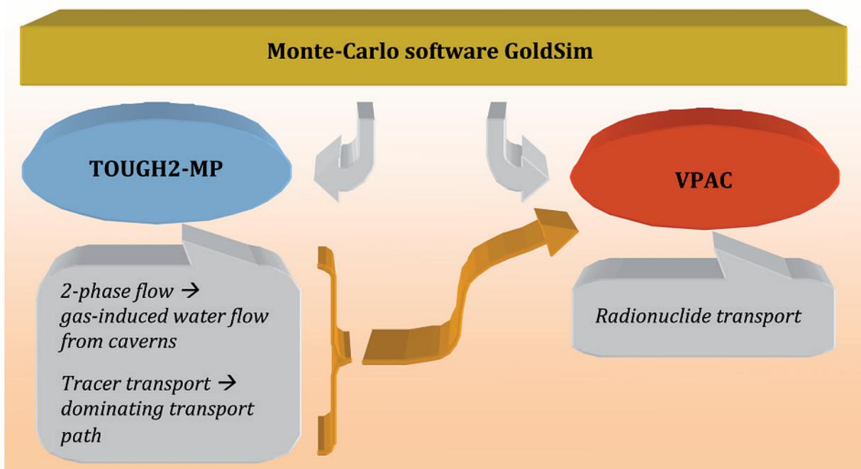
**Figure 1:** Model chain of the probabilistic radionuclide transport calculations.
